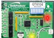
If the **Yellow** LED is off, verify power to the Qwik**Swap**® board. If the **RED** LED is off or flashing, there is a communication error.
