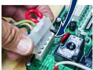
5-pin Connector from Motor to Qwik**Swap**® Board
