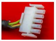
**No Jumper Wire -**Set Azure® motor for 240V operation
