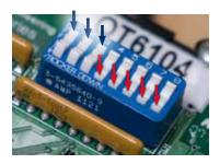
In this figure the motor has been set to 1/3 hp: (ON, ON, ON, OFF, OFF, OFF, OFF, OFF)
